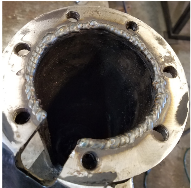
Fig. 3: Spot welds around flange circumference
