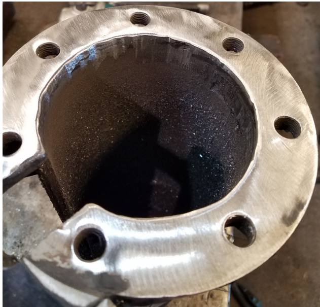
Fig. 5: Flange restored to its original inner circumference profile
